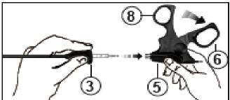
Insert the shaft tube with the jaw part into the handle (5) in the direction of the arrow. The tube part and the assembled jaw part can only be inserted into the handle if the jaw part and tube are correctly placed one inside the other. Note the color marking at the end of the pipe! Turn the knurled nut (3) in the direction of the arrow and tighten slightly.
