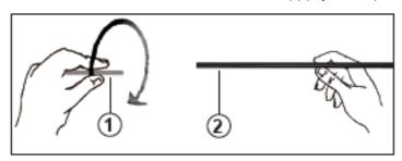
The dismantled instrument then consists of three parts: jaw part, shaft tube, handle. Instruments with metal handles are disassembled in the same way.
